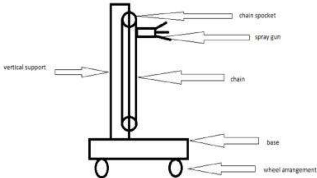
**Figure : Basic Structure Of Wall Painting Robot**
